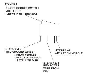
Terminals on switch have to be bent to fit in surface mount box.
